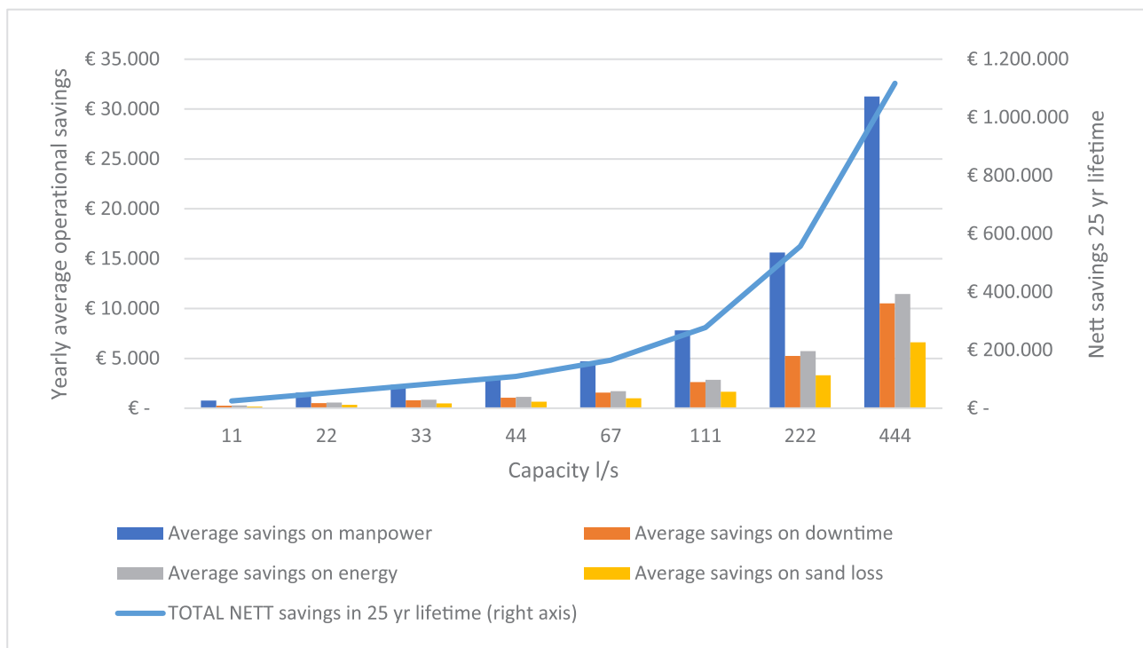
Figure 5 Estimated savings per parameter for 8 plant sizes based on their capacity (l/s).
