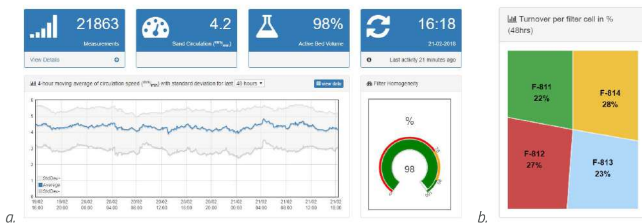
Figure 3 (a) The dashboard illustrating the number of RFID tag responses, sand circulation (mm/min), active bed volume, last activity, 4-hour moving average sand circulation speed (mm/min) with standard deviation for last 48 h time period and filter homogeneity (b) the turnover per filter cell displayed at WwTW Franeker
