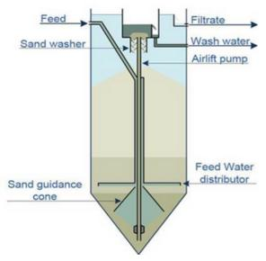
Figure 6 – Schematic of Continuous Sand Filter
