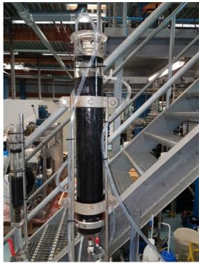
Figure 5 – Lab trials - GAC Column Tests
