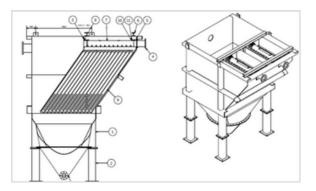
Figure 3 Tilted Plate Settler
