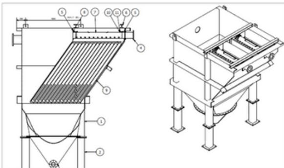
Figure 3 Tilted Plate Settler
