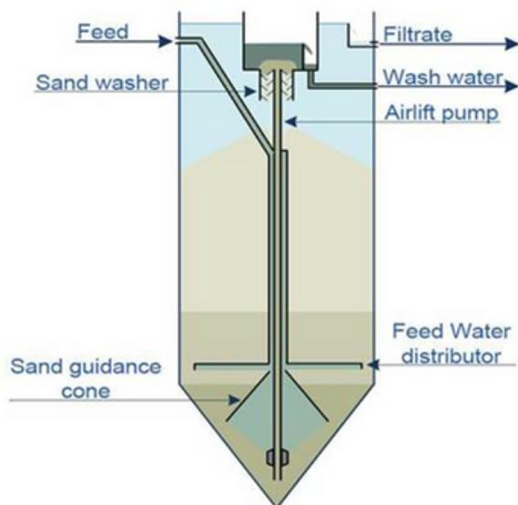
Figure 6 – Schematic of Continuous Sand Filter
